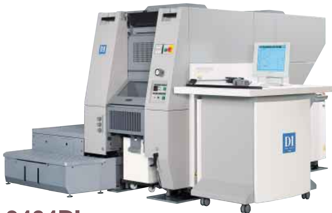
RYOBİ 3404DI A3-Size Portrait Format 4-Color Offset Press with Built-in Direct Imaging
