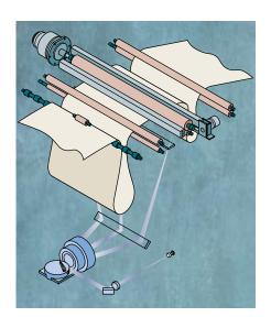
Inside the FT-Rs a diode-generated laser beam is reflected onto the imaging media by a multi-facet polygon mirror rotating at high speed. A specially designed lens eliminates the effects of any wobble in the imaging system, though very little is generated to begin with, thanks to high-precision machining and components.
